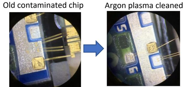
In the photos above, argon plasma cleaning makes the tarnished silver pads look brighter and shinier after the surface organic contamination and silver oxide layer are removed. The data below shows that the pull force for the wire bonds significantly improved after 3 minutes of pure argon plasma cleaning.
