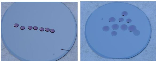
Water droplet contact angle on chip package before and after argon plasma cleaning (external link to a youtube video)
